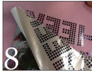
**VERY IMPORTANT:** Rub with a cloth, allow to cool completely before removing foil sheet.
