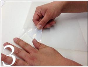
Cut out around your plotted designs and weed the excess from the carrier. The sticky carrier makes it easy to re-stick small details that might pop up during weeding.
