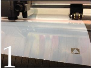
Load roll so the material is rolled out from underneath. Use a 45° blade with very low pressure. Do a cut test until the outer shape weeds out easily around the inner shape.
