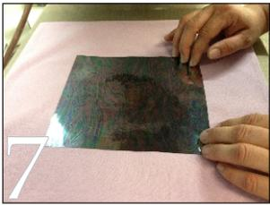
Carefully place foil over the HotMelt design and make sure it completely covers it. Heat set at 300°F for 10 seconds.
